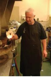
lemel being melted and then immediately place the melted button into the X-ray machine, which gives the customer a rough on-the-spot assay. This means the customer has a rough idea of what assay to expect and is safe in the knowledge that the process is as transparent as it can be.
